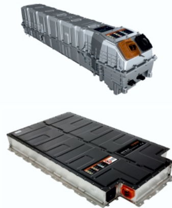
BMW HV battery 10 / 40 kWh 350V
